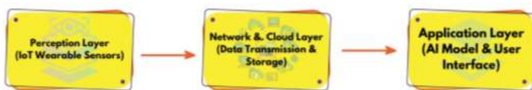
Figure 2. System Architecture of AI-Driven IoT Pet Healthcare Framework
